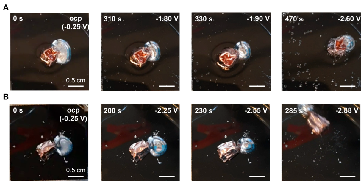
Figure 5.8. Snapshots of voltage-driven reactions between bulk liquid Ga and Cu which mimic the dimer configuration. Images at selected time points representative of the bulk liquid Ga – Cu “sphere” mimicking the nanodimer in the bulk during cathodic linear voltage scan at (A) 5 mV/s and (B) 10 mV/s.
