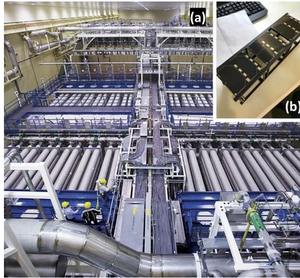
Figure 3 - Two lasers of very different scale: a) The 48 beamlines comprising the United States National Ignition Facility (" Seen from above " by U.S. Department of Energy is licensed under CC0 1.0 .) and b) a typical 3U-cubesat (30 cm x 10 cm x 10 cm) into which a laser may be installed. A computer keyboard is visible as a point of reference (" 3U Cubesat with solar panel PCBs mounted " by AphelionOrbitals is licensed under CC BY 2.0 .)
