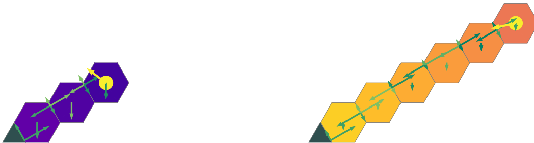
(a) When only three blocks need to be held, the force received by each is quite small compared to the maximum force of the robot, so the color remains uniform.
