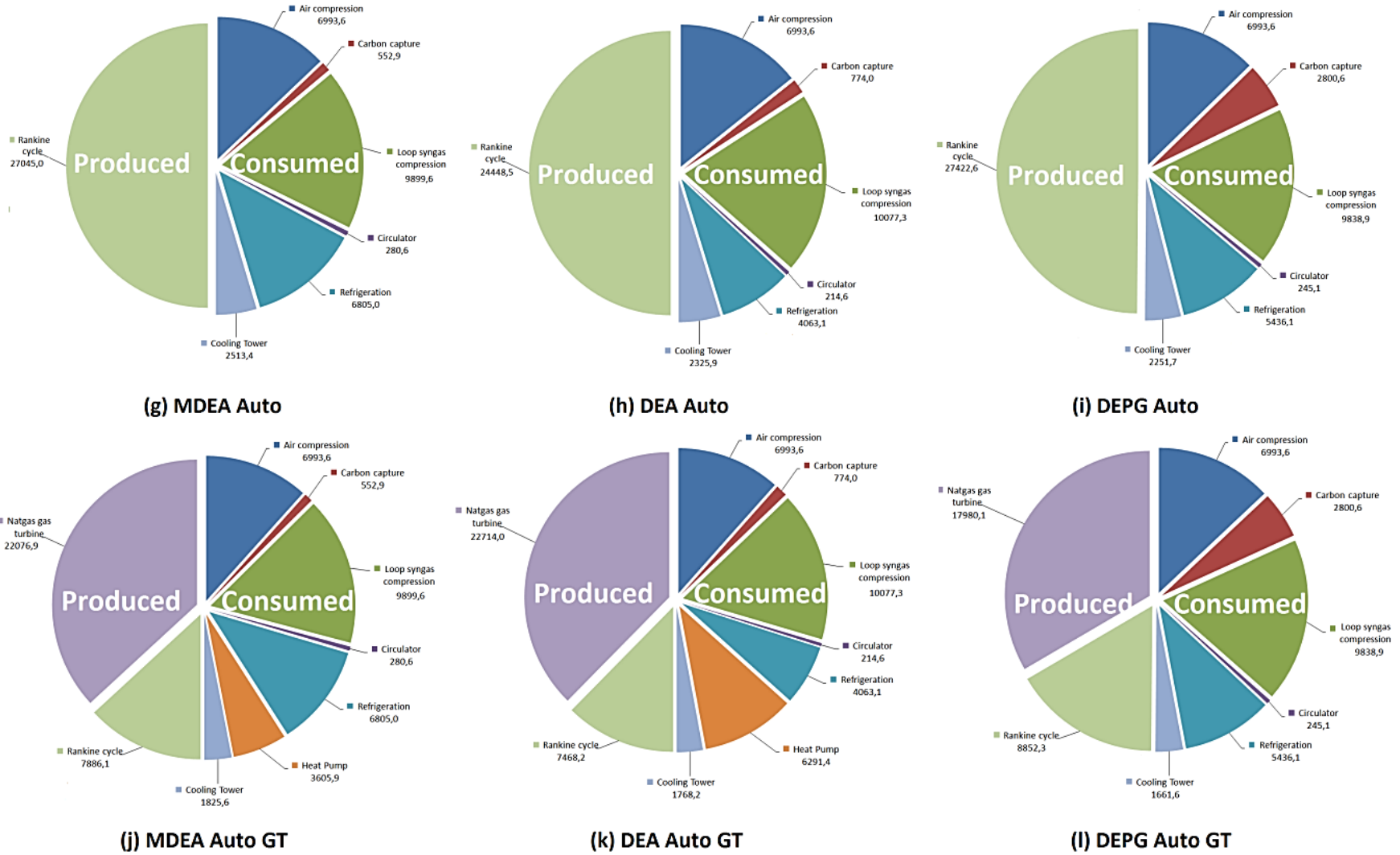
Fig. 7.8. Breakdown of power generation and consumption in each plant configuration shown in Table 7.2. (cont'd). Source: Author
