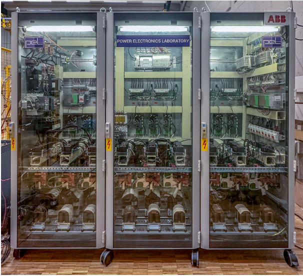
Fig. 2. The Power Electronics Traction Transformer (PETT), analyzed as example of an ISOP SST: Top) Circuit Topology; Bottom) Experimental setup.
