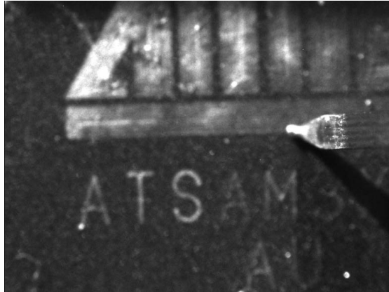
Figure 2.3: Position of an EM microprobe on a SAM3X8E Cortex-M3 microcontroller at which strong EM radiations could be collected.
