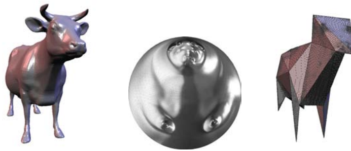
Figure 8.4: Mapping a cow model (left) to the sphere (center, using [ZRS06]) and to a base triangulation (right, following [LSS+98]). The maps are visualized by the original shading and original vertices in coarse base triangles, respectively.
