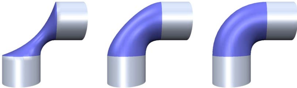
Figure 7.3: The order k of the energy functional and of the corresponding Euler-Lagrange PDE \Delta_S^k \mathbf{x} = 0 defines the stiffness of the surface in the support region and the maximum smoothness C^{k-1} of the boundary conditions. From left to right: membrane surface ( k = 1 ), thin-plate surface ( k = 2 ), minimum variation surface ( k = 3 ).
