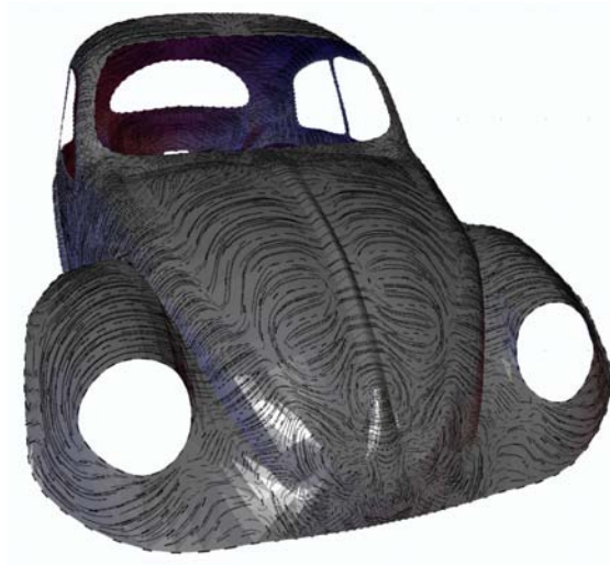
Figure 6.5: Lines of curvature. Lines of curvature are superimposed on a flat shaded image of a VW Beetle model.
