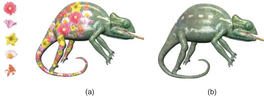
Figure 4.12: Editing operations on the Chameleon (101,685 points): (a) texture painting, where the flowers shown on the left have been alpha-blended onto the surface, (b) texture filtering, where an oil-paint filter has been applied to the left half of the model.
