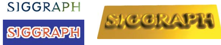
Figure 3.12: Embossing effect. The Siggraph label on the top left has been converted to a selection stencil using simple image processing tools. This stencil can then be mapped to a surface, where blue color corresponds to the zero-region and red to the one-region. Subsequent deformation yields an embossing effect as shown on the right.
