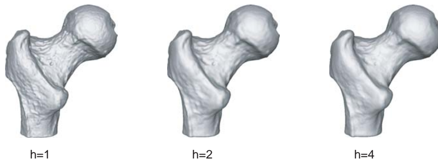
Figure 1.4: Smoothing effect of the MLS projection. The Gaussian kernel width has been doubled for each image from left to right.
