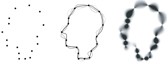
Figure 1: A given point cloud (left image) could be a sample from any of an infinite number of surfaces. In the middle, four such surfaces are shown, where the gray value indicates the prior, i.e., likelihood that the point cloud is sampled from this surface. The accumulated likelihood for all surfaces as computed with our method is shown on the right.
