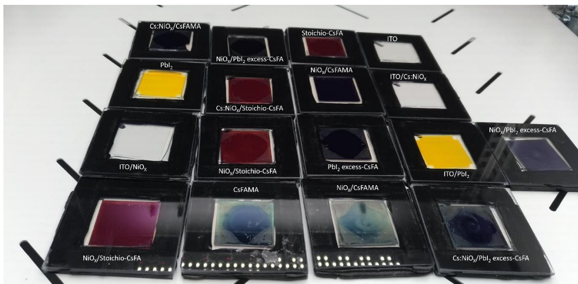
Figure 5.1: Picture of the Different Samples in the Cicci Chamber at Room Temperature under LED Arrays.
