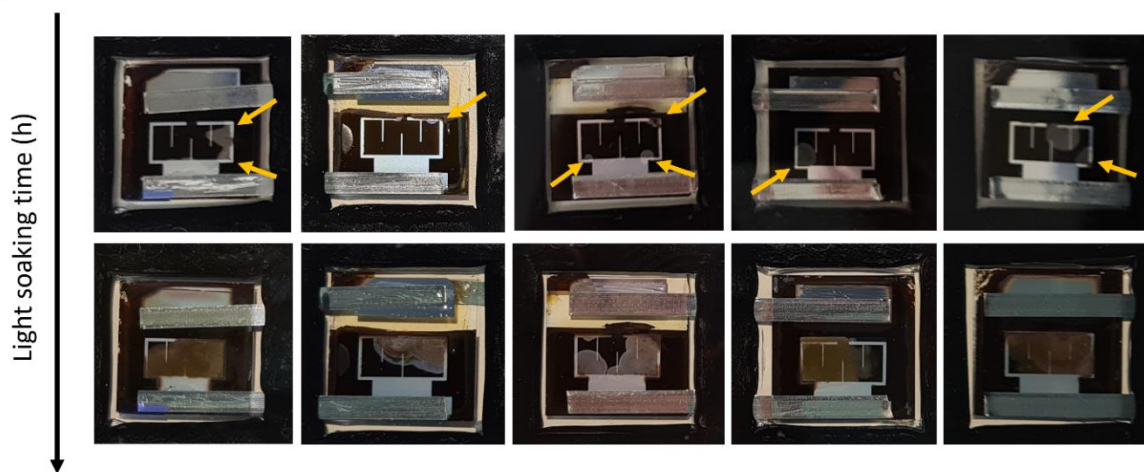
Figure 5.12: Encapsulated Cells After > 400 h of Substrate Side Light Soaking at 65°C and at V oc in the Solaronix Chamber. Stack: glass/ITO/NiO x /(SiO x )/CsFAMAPb(I 2 Br) 3 + pFBPA/C 60 /SnO 2 /ITO/Ag.
