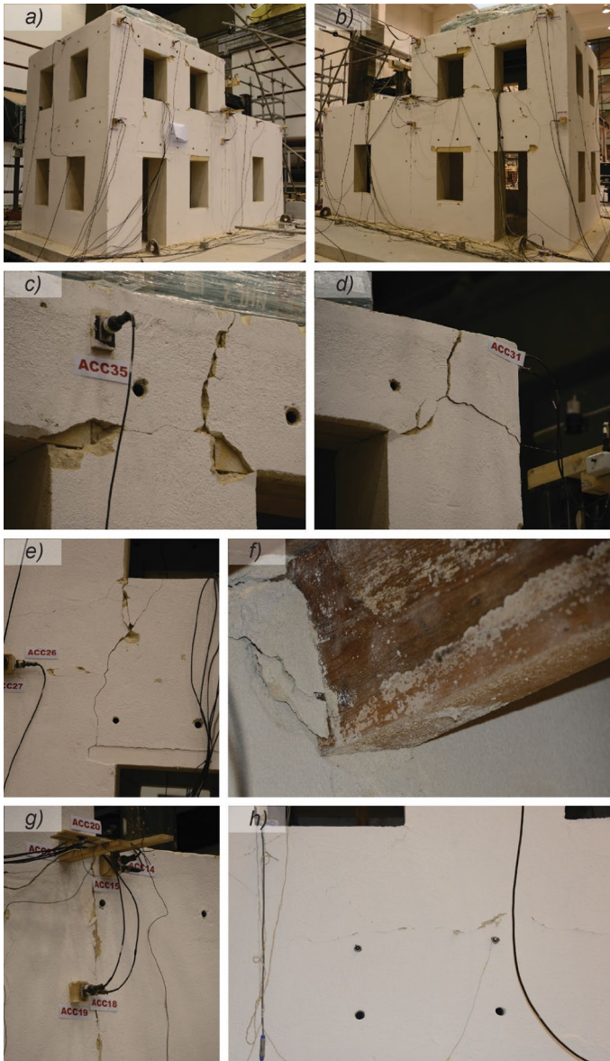
Fig. 17 Damage observed at the end of test run 2.1: a-b External view of the aggregate; c Flexural cracking of a 2nd floor spandrel and at the top of a 2nd storey pier of Unit 2; d Cracking and near-detachment of the top of a 2nd storey corner of Unit 2; e Flexural cracking of a 1st floor spandrel of Unit 2; f Slip of a 2nd floor joist of Unit 2; g Damage at the interface between the units; h Horizontal crack at the 1st floor level of facade 4 of Unit 2
