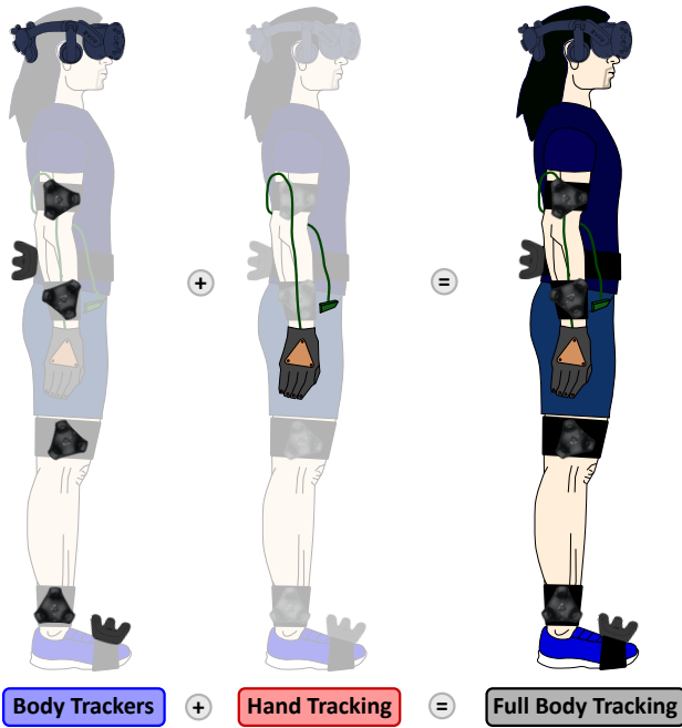
Figure 3: The setup involves a mix of Vive Trackers 3.0 with home-made tracking gloves, therefore mixing tracking solutions.
