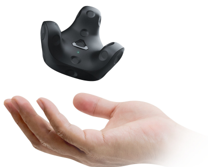
Figure 1: Vive Tracker 3.0 is a consumer-grade device whose 3D localization can be retrieved through SteamVR. Those trackers are well suited for the gaming experience, for tracking limbs (e.g., feet, knees, etc.) or objects to interact with (e.g., tracking a dummy gun). However, their dimensions prevent them from being placed on each finger.
