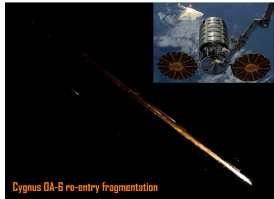
Figure 2.2: Cygnus OA6 re-entry fragmentation picture taken from the dedicated observation aircraft.[10]. Spacecraft image credit: NASA [11].
