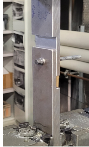
Figure 3.15: Single shear setup to evaluate for M5 bolt shear strength.
