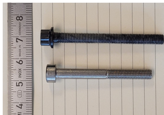
Figure 3.2: Baseline stainless steel versus our novel CF/PEEK bolts for through-thickness insert fixture to a sandwich panel.
