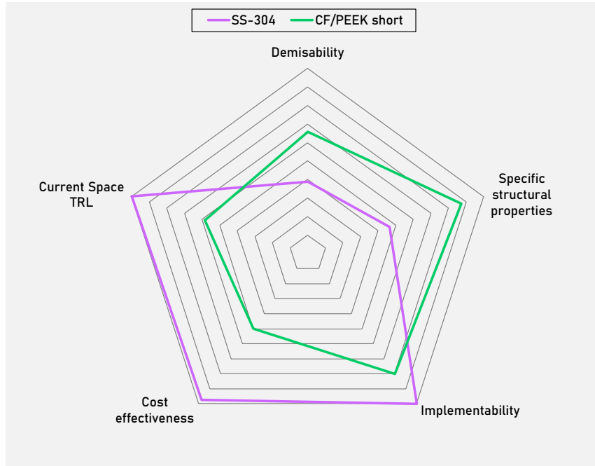
Figure A.10: Radar plot of the SS and short-CF/PEEK fasteners as function of 5 D4D dedicated indexes.
